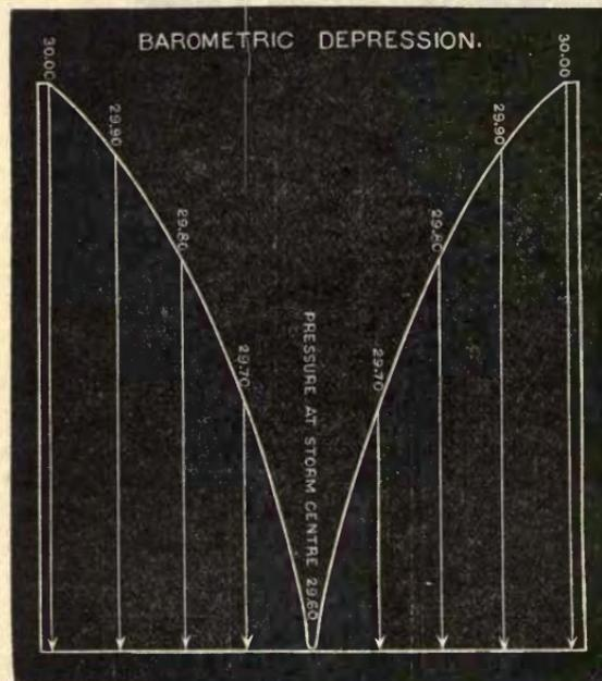
Diagram of pressure in a section of a cyclone.
