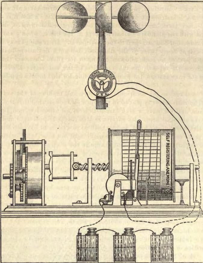
Signal Service anemometer, with self-registering attachments.
